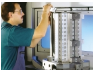
1. The clamping module with its eccentric lock released is inserted in the high-precision slot
